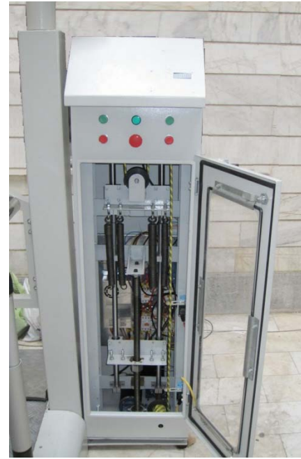
Fig 4. The body weight support system constructed for LOKOIRAN rehabilitation device
